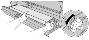
**9** Rotate the roll holder in the direction of the arrow, then cut the media along the edge of the paper guide.
